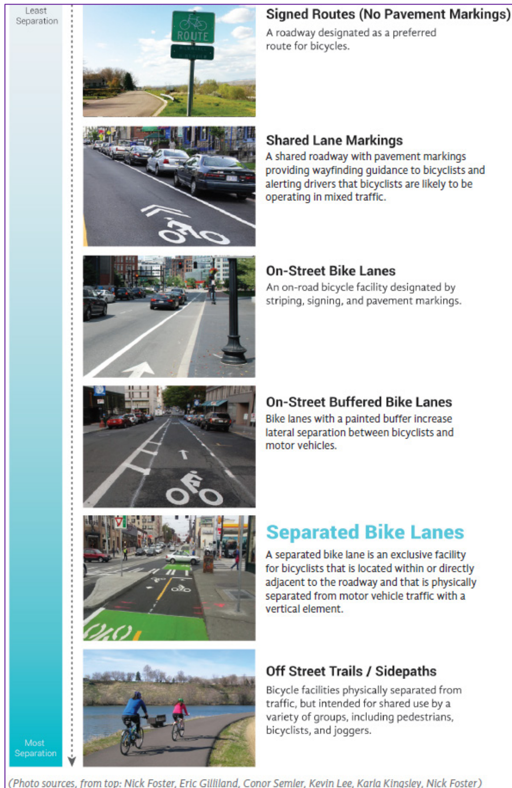
Figure 2-1: Degrees of Bike Lane Separation
